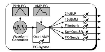
Directly next to the sound-source (Waveform Generation) there is an amplifier (triangle-symbol), which is controlled by an envelope. The level controls for the individual filters come after it! Below the amp you will see the "EG-bypass-signal path". This one routes the signal of the current waveform directly to the output volume pots - just bypassing the volume envelope.
