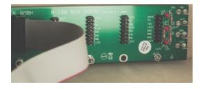
Once you have connected the cable, you can place the module in the correct position and install it using the enclosed screws and washers. Please use the plastic washers - so you can exclude damage to the painting and silkscreening.
