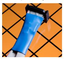
Now take the ribbon cable and insert the side with the shrink-tube insulation into the 16-pin socket of the DSP board. The 16 pin socket is easy to recognize. Make sure that the DSP board is not exposed to unilateral pressure while inserting the cable into the IDC plug, and that the circuit board connectors between the DSP board and the Frontpanel board remain connected.
